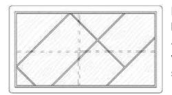
Install a second layer of plywood on top of the first layer, also made of entire sheets, but at an angle of 45° relative to the first layer. This will give to the whole structure additional rigidity, strength and stability.
