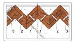
Start installing the base elements from the center line along the wall farthest from the entrance. Do this by "dry" method - without fixing it with glue, to check the correctness of the laying and ensure accuracy before final fixing.
