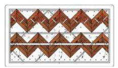
Draw a line with a marker using a straightedge set exactly at the tops of the inside corners of the first row of planks. This will be the starting line after the boards are cut and laid into the overall covering. Number the boards to avoid mistakes when laying them out. Cut the boards along the markings. Use
