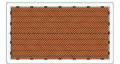
Continue laying to the opposite wall, remembering to install spacers along the walls. Once installation is complete, use the remaining pieces of parquet cut at the beginning. Clean the parquet from debris and dust using suitable care products.
