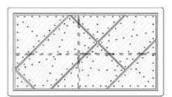
Use mechanical fixation to securely fasten the plywood between the layers. Place the fasteners around the perimeter of the sheets at intervals of 10 cm and additionally diagonally for better connection of the layers. The length of the fasteners should be less than the total thickness of the plywood layers,
