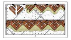
Install spacers along the wall to create a compensation gap. Apply glue to the base. Start laying the boards from the center line, alternating rows on both sides of it. Tap the boards with a hammer through the spacer so that the tongue fits tightly into groove, without gaps. To secure the
