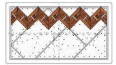
Make sure that each row is laid out evenly and fits tightly against the previous one. Check regularly for proper installation and expansion gaps. Make sure that everything is flat.
